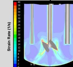
Spatial distribution of strain rates in 2-L stirred tank bioreactor.
