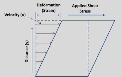
Figure 1. Schematic Illustration of Fluid Shear
