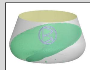
Predicted air-liquid interface in 2-phase shake flask model.
